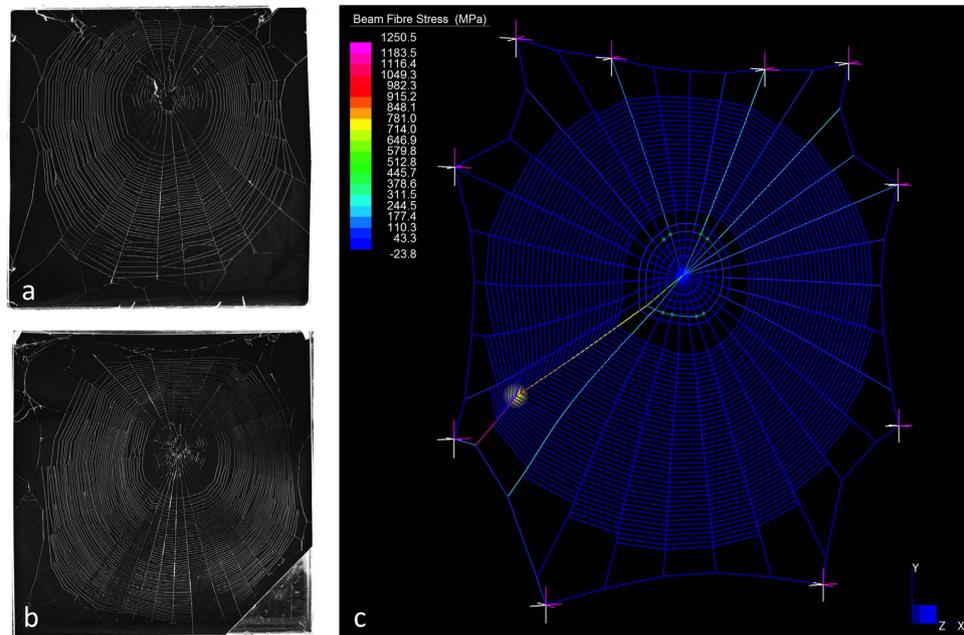
**Figure 4.** Example webs built in small and large frames and example finite element model. (a) Web built in a 25 × 25 cm frame. (b) Web built in a 50 × 50 cm frame by the same spider. (c) Finite element model of an average web built in a 50 × 50 cm frame.
